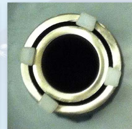
**Figure 2:** The smaller the gap between the outer (cathode) and inner (anode) tubes, the stronger the force.
