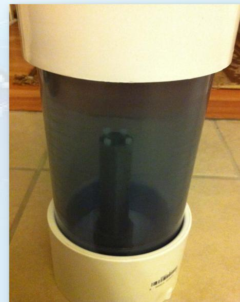
**Figure 1:** The Generation Chamber consists of a 18" section of 4" Clear PVC tubing, capped by a PVC cap and the electrode wires. A flow rate meter is attached to the top to measure the quantity of Hydrogen gas being produced.
